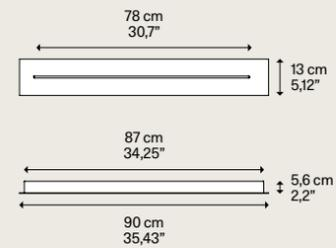
Net weight 7,33 kg / 16,16 lbs | Boxes Colli 1 | Connectable directly to a 4" Standard J-Box
