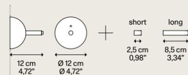
Net weight 0,40 kg / 0,88 lbs | Boxes Colli 1 | Mounts directly to a 4" Standard J-Box
