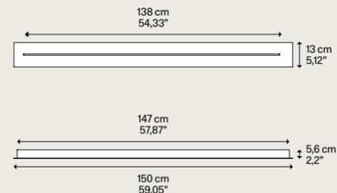
Net weight 11,85 kg / 26,12 lbs | Boxes Colli 1 | Connectable directly to a 4" Standard J-Box
